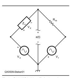
Fig 1—Old LMS bridge. Zx is the unknown and Rm is reference resistor.
