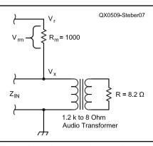
Fig 7— Setup for measuring transformer or speaker impedance.
