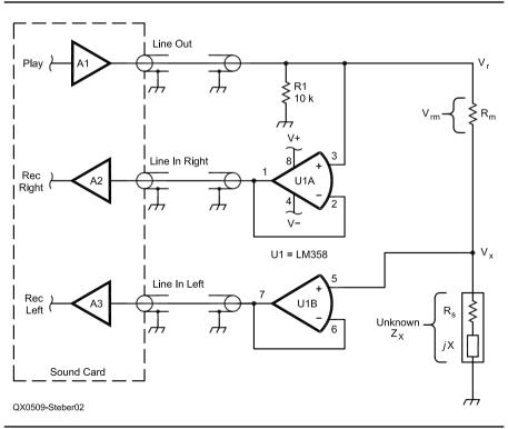
Fig 2—Impedance measuring circuit and interface to sound card. See text for more information.
