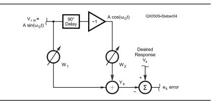
Fig 4—An adaptive combiner for the LMS bridge.
